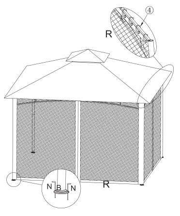
Step 8:Insert the stakes(Part N) on the foot pad to the ground deeply, use Part (4) (the plastic hook) to hang Part R on the frame,then you can use the gazebo.
