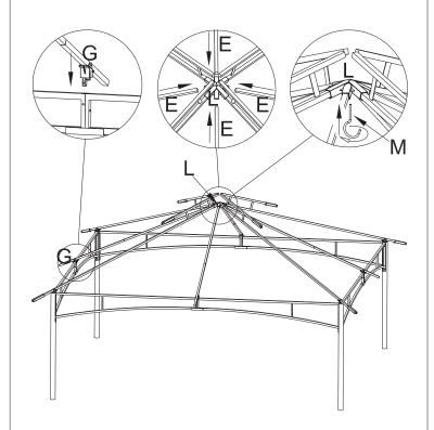
Step 5:Insert Part G to the middle part of the two attached part C. The other three Part G should be done as this. Then insert the other head of Part E to Part L. Finally, Insert Part M(the steel hook) to the hole of Part L and turn it to tighten it.
