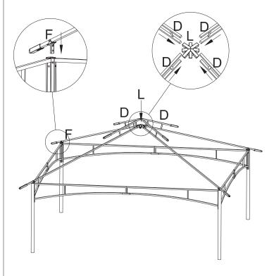
Step 4:Insert four Part F to the four corners of the frame (the top of Part A) . Then insert the other side(the bottom side of Part D) to Part L.  $\boxed{4}$
