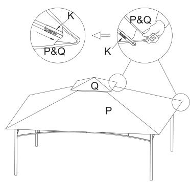
Step 6:Put the canopy fabric (Part P&Q) on the frame, extend it fully. Put the heads of tubes(Part K) into the corner pocket of canopy fabric.
