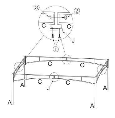
Step 2:Use Nut③ and Srew② to connect two Part C and tighten them.
